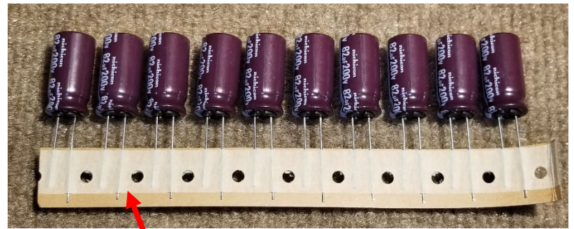
Peel tape off positive leads. Do not cut them.
